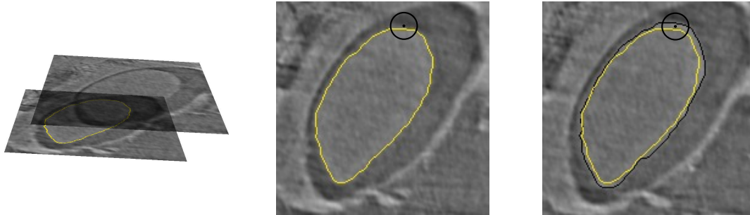
Figure 6: Active contours slice by slice. Left : Use prior segmentation as initialization and move forward in z -direction. Center : Slice n with related solution. Right : Slice n + 1 with initialization (yellow) and final solution (black). The circle represents a local region A(x, y) at position x . In step n , x lies outside, in step n + 1 , x lies inside the contour.
